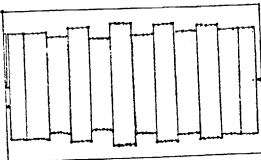
Figure 2 Considerable runout. NOTE: If this condition exists ensure that mating of spindle and disk are clean. Improper mating can cause such runout.
